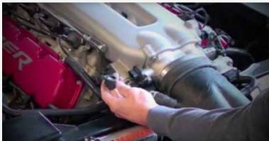
Disconnect the throttle cable from its tab by pulling forward on the black cable end.
