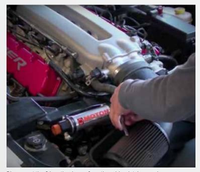
Disconnect the 2 breather hoses from the rubber intake coupler.
